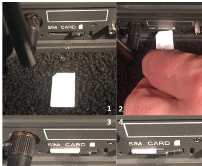
Figure 2-5 Installing SIM Card and Engaging the Lock
