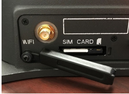
Figure 2-4 SIM Card with Cover Opened
