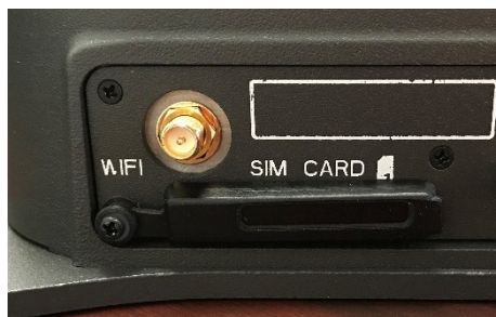
Figure 2-6 Secure the SIM Card Cover
